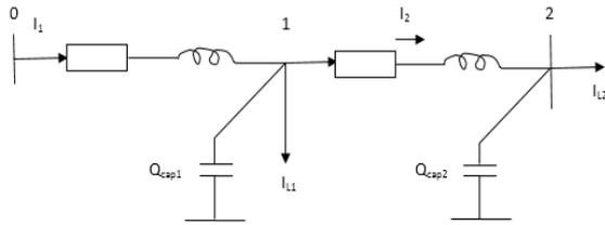
**Figure 3: Impedance diagram of Okesa feeder with the proposed positions of compensating capacitors.**
