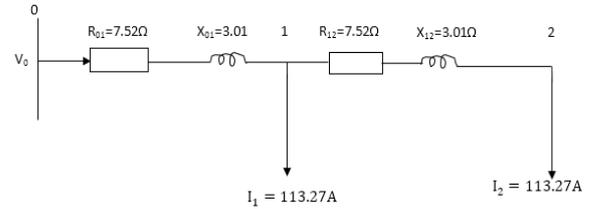
**Figure 1: Impedance diagram of Okesa Feeder when half feeder load is at the middle and the other half is at the end of the line**
