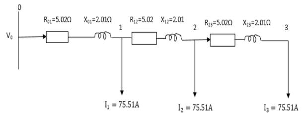
**Figure 2: Impedance diagram of Okesa feeder when the load is distributed equally**
